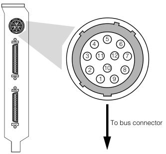
Figure 21. Pin numbering for Hirose HR10 connector
