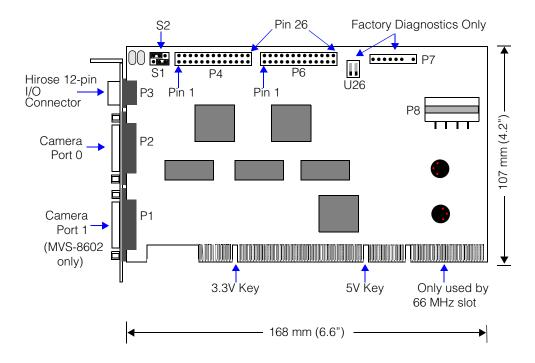
Figure 15. MVS-8602 component location diagram
