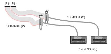
Figure 10. General-Purpose I/O Kit Components
