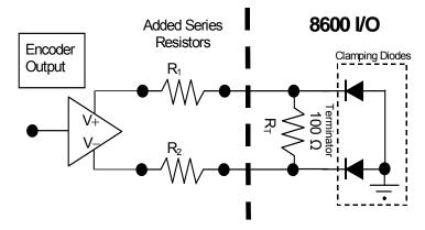
Figure 29. Schematic with series resistors
