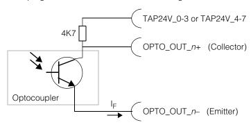
Figure 26. Opto-isolated output circuitry for programmable lines
