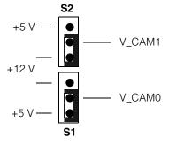
Figure 18. Default settings for MVS-8602e S1 and S2
