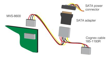
Figure 5. SATA adapter and power adapter cable
