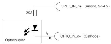
Figure 25. Opto-isolated input circuitry for programmable lines
