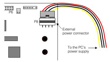
Figure 4. Connect power supply cable
