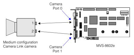
Figure 7. Medium camera connection example
