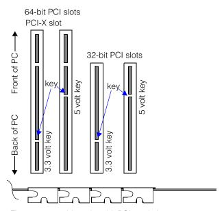
Figure 1. 32-bit and 64-bit PCI card slots
