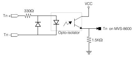
Figure 27. Schematic for opto-isolated trigger input on I/O connection module
