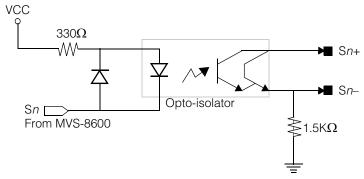
Figure 28. Schematic for opto-isolated strobe output on I/O connection module
