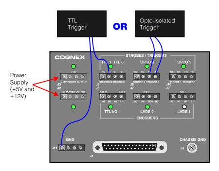
Figure 11. Trigger wiring for I/O options 1 and 2
