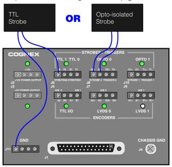
Figure 13. Strobe wiring for I/O options 1 and 2
