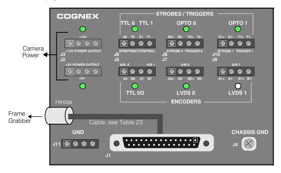
Figure 24. Wiring connections on I/O Connection Module
