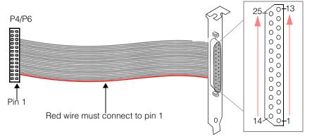
Figure 9. I/O extension cable, Cognex part number 300-0240
