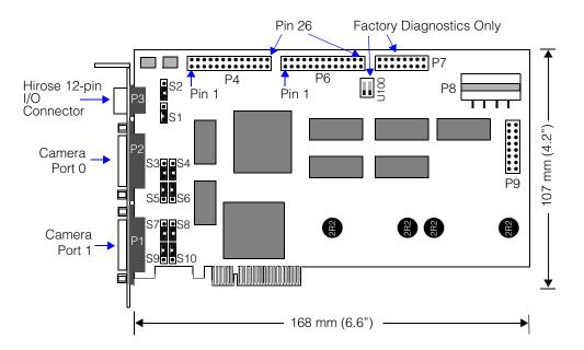
Figure 16. MVS-8602e component location diagram
