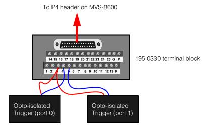
Figure 12. Wiring triggers for I/O option 3
